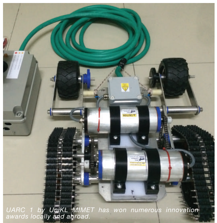
The amphibian rover which is fitted with a camera can travel on land and in water efficiently
